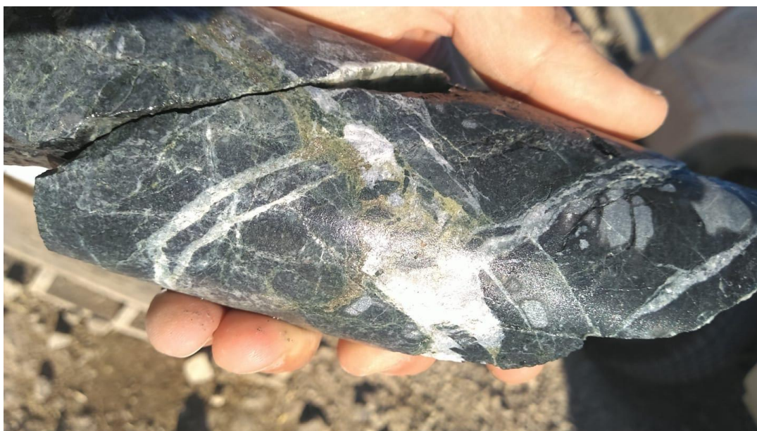
Figure 3 – 19VNDD001 (299.6m). Mineralisation as blebs and disseminated grains of pyrite and chalcocopyrite associated with coarse-grained epidote and calcite
