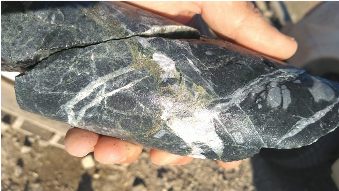
Figure 3 – 19VNDD001 (299.6m). Mineralisation as blebs and disseminated grains of pyrite and chalcopyrite associated with coarse-grained epidote and calcite
